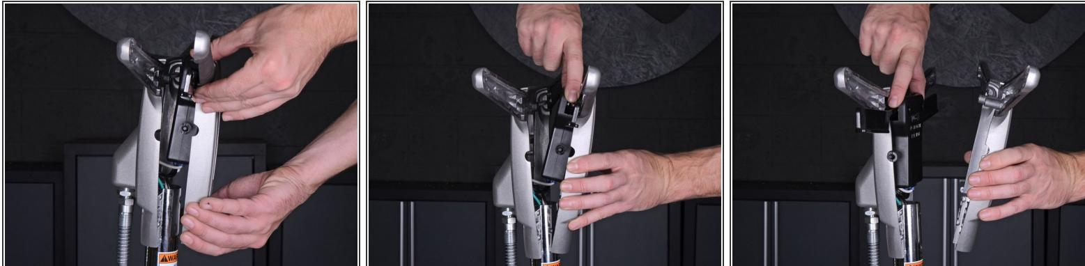
**(i)** The rear half of the enclosure is bolted to the handle support, so the front half will be removed first.
