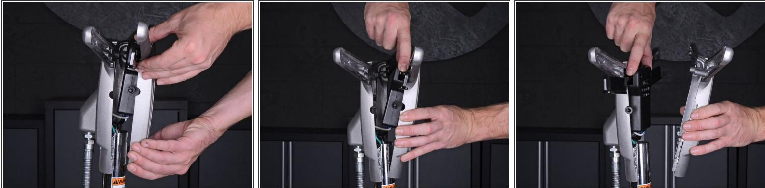
ⓘ The rear half of the enclosure is bolted to the handle support, so the front half will be removed first.
