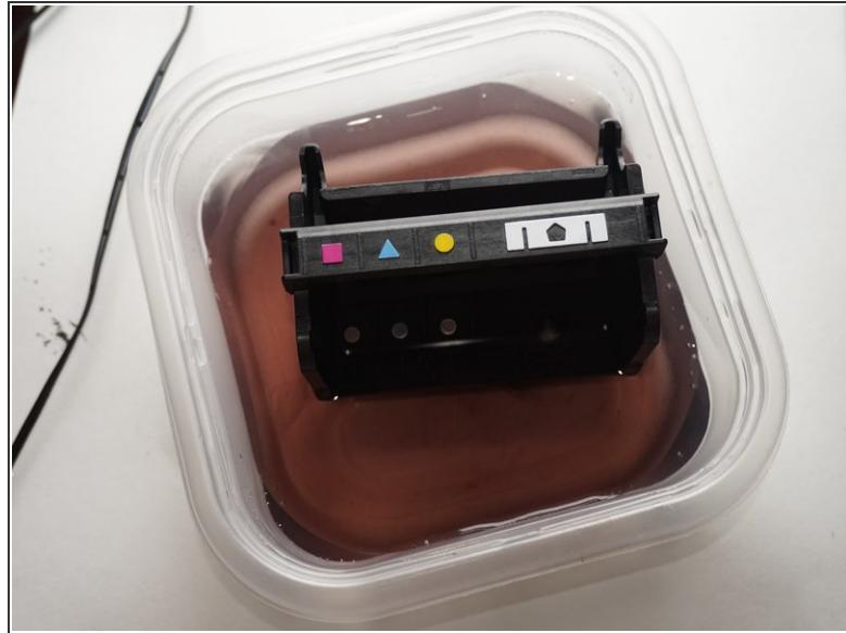
**⚠ Do not use alcohol unless you are out of options. This may damage the printhead! Purge the printhead 3 times if alcohol is used to avoid problems.**
