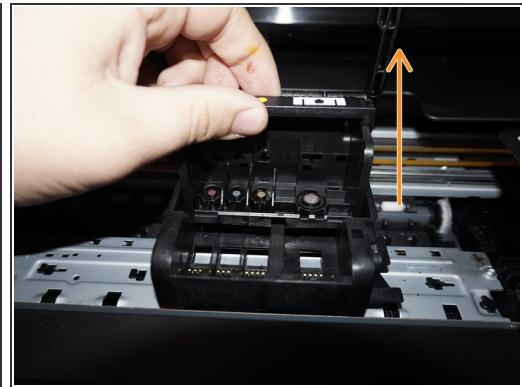
**⚠ If the printer is plugged in while the printhead is removed, the calibration data may be erased. Verify the printer is unplugged BEFORE removing the printhead.**
