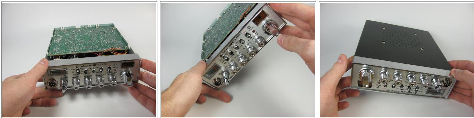
**⚠** Gently set down on a hard, flat, non-conductive surface to minimize risk of shock or breaking your radio.
