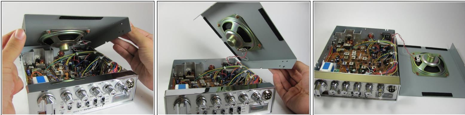
**⚠** Watch out for the wires connected to the speaker. These short wires will not allow you to move the cover very far.
