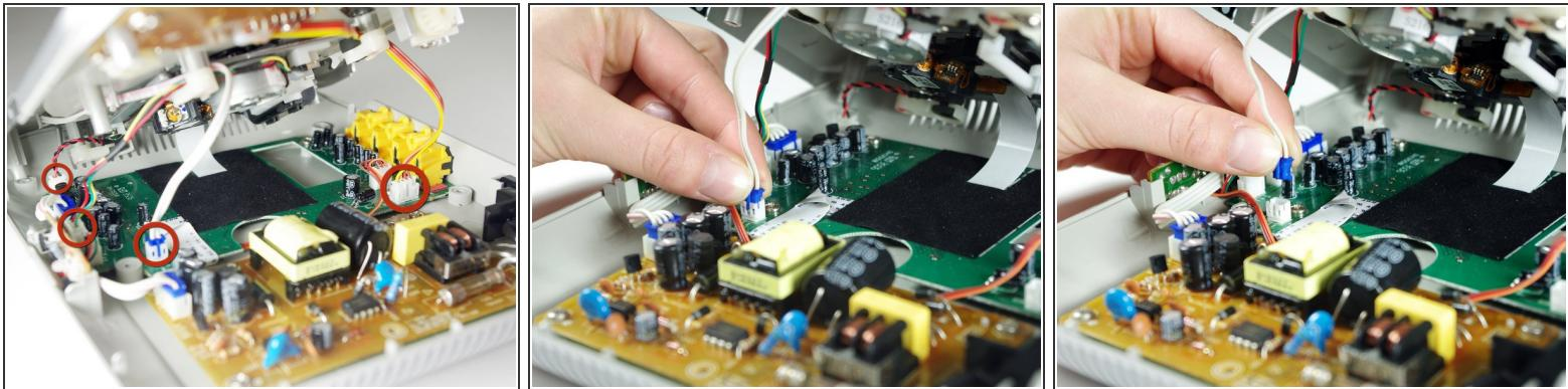
**⚠** When pulling the ribbon cables out, make sure not to pull by the wires, as this can cause damage to them.
