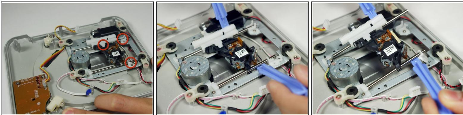
**!** There are three small 4.5mm springs that can be easily lost. Be careful when lifting up the railing assembly to make sure you don't lose them.
