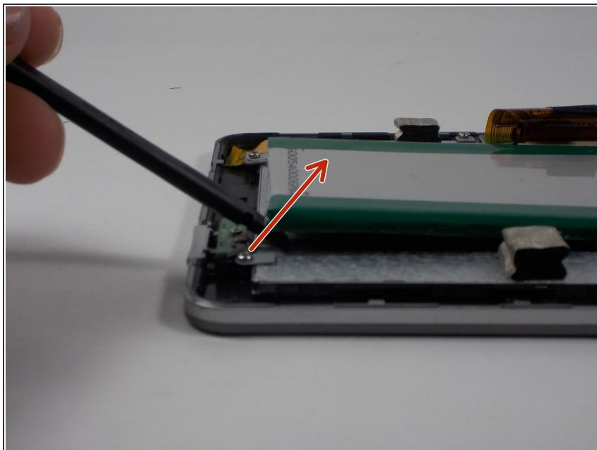
**!** Knowing the location of the ribbon cable, use plastic spudger to pry off battery.
