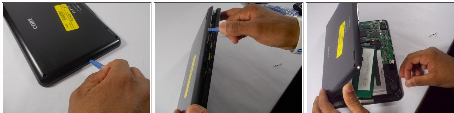
⚠ Be careful not to break the inner plastic tabs while pulling the back cover off.
