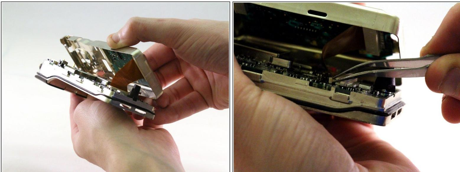
*(i)* The keypad chip is attached to the motherboard by a ribbon.
