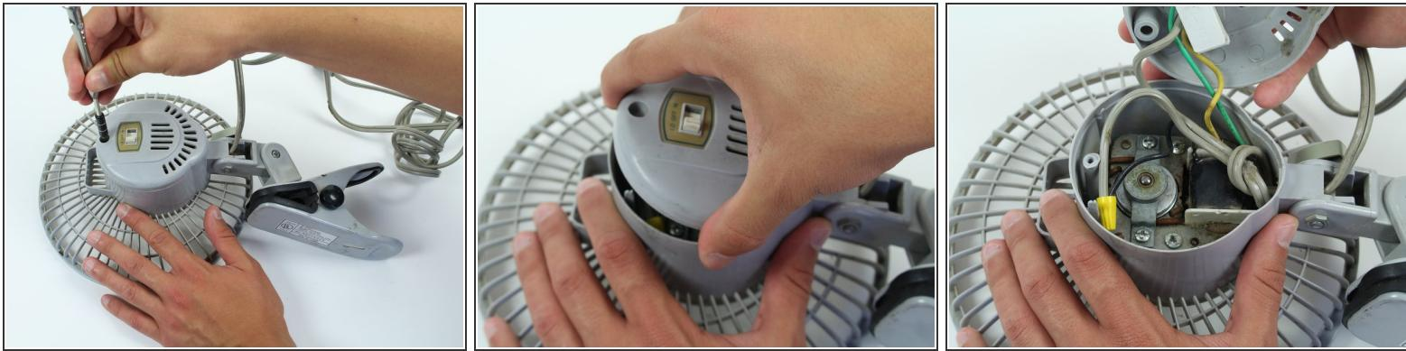
**⚠** Make sure to unplug the Comfort Zone CZ6C before cutting any wires.
