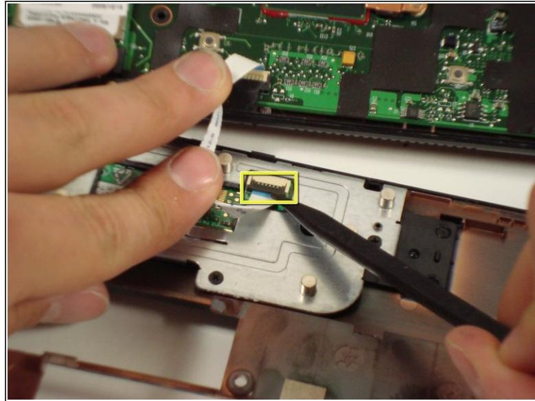
! Careful lifting up the cover because the track pad is still attached.
