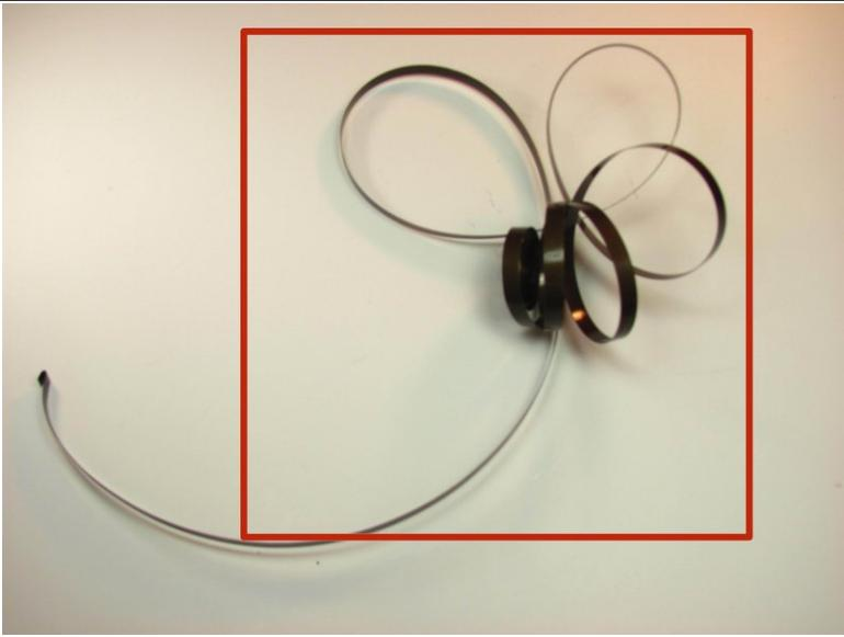
**⚠** When removing the coil, make sure it stays wound up. It could very easily pop out, and you would have to wind it all the way back up and try to squeeze it back into the slot when you reassemble the dryer.
