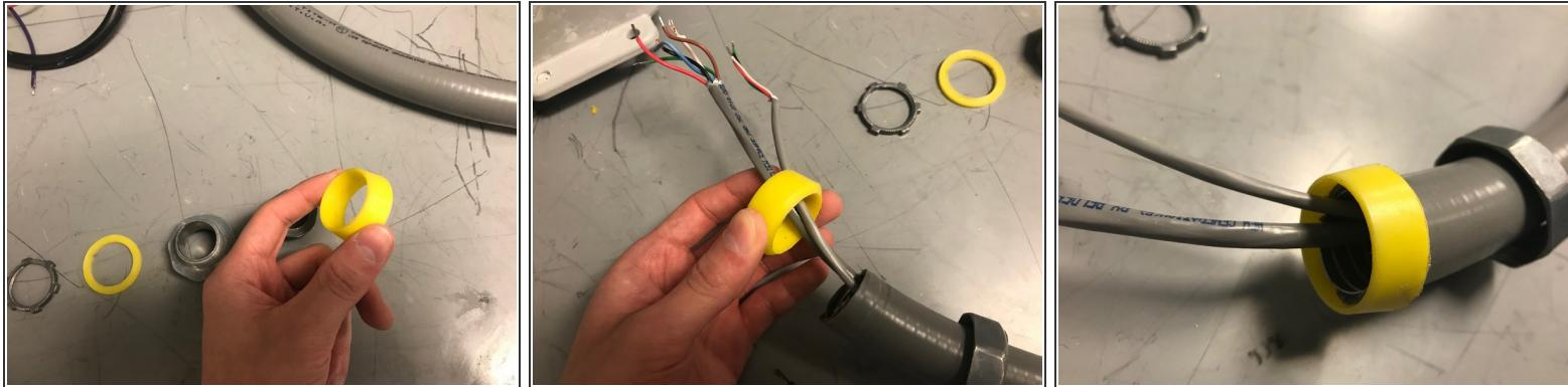
① Pull the outer yellow seal over the wires and the conduit
