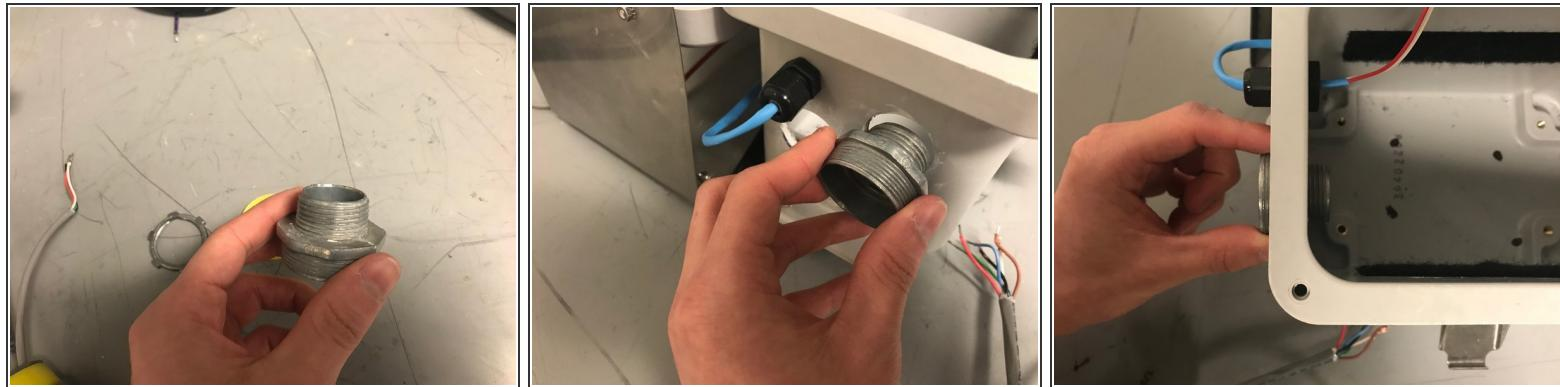
① Put the connector piece into the node (may have to hold it in place for the subsequent steps)
