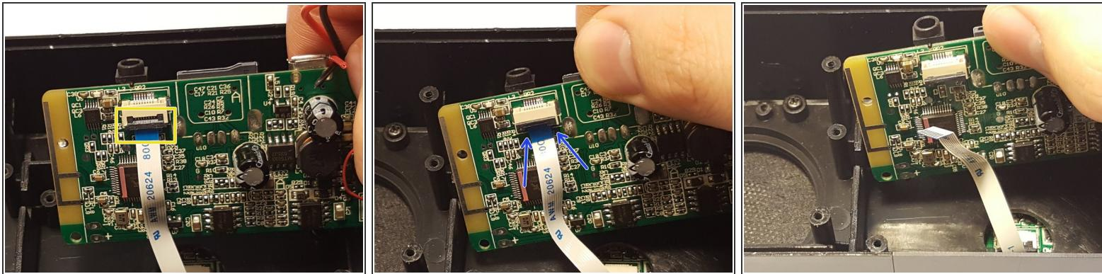
*(i)* You will finds a ribbon connecting the motherboard to the control interface circuit board.
