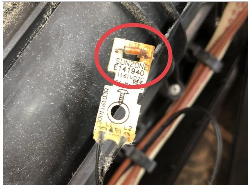
*(i)* The temperature sensor had broken because it was corroded by moisture and therefore rusted.
