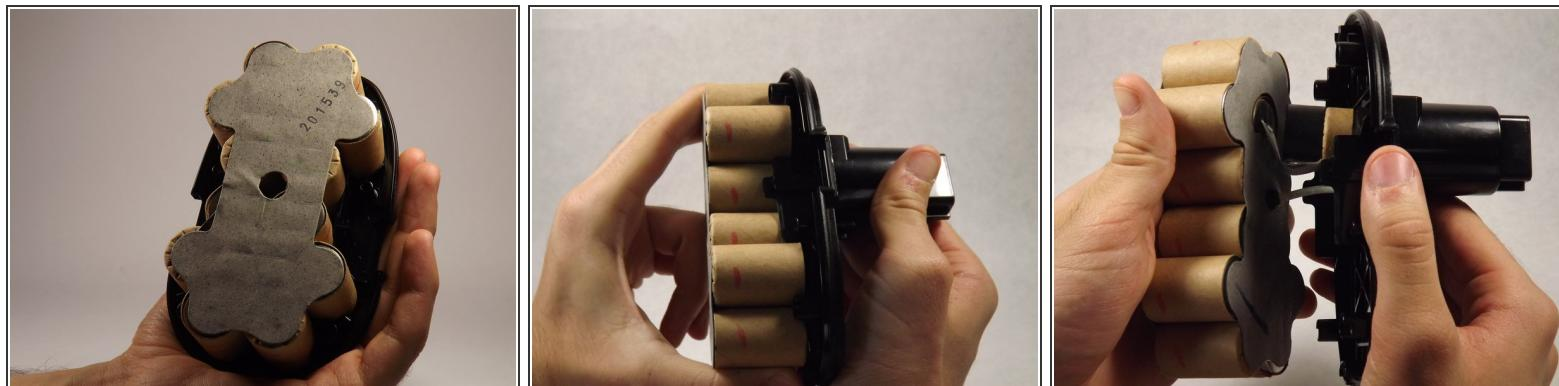
**⚠** Remove the old battery cells by slowly pulling them out of the top piece of the battery.
