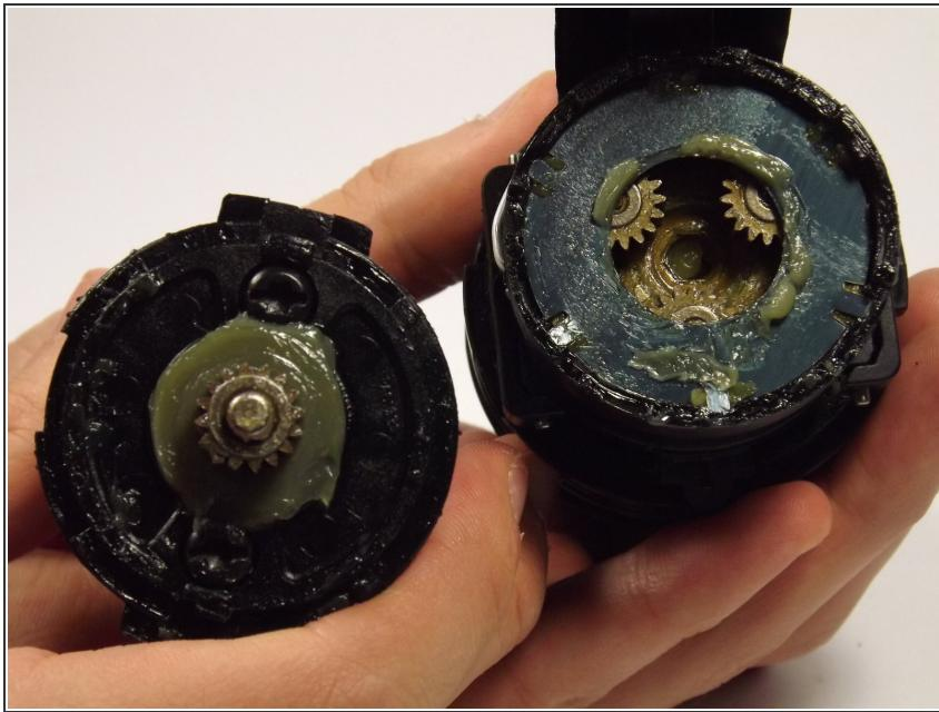
When installing the replacement motor into the clutch make sure you correctly align the gears in order to assure that the motor is properly fitted to the clutch.
