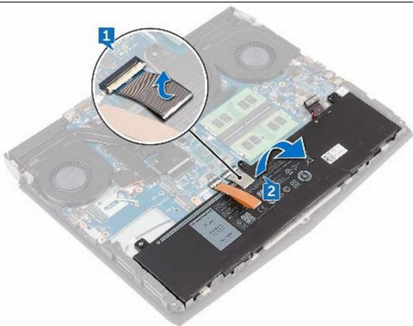
**⚠ CAUTION:** Ensure the keyboard and keyboard-backlit cables are not under the battery.
