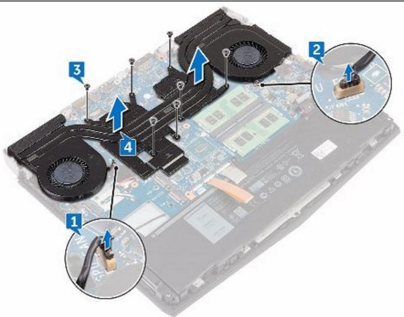
**!** CAUTION: Incorrect alignment of the heat sink can damage the system board and processor.
