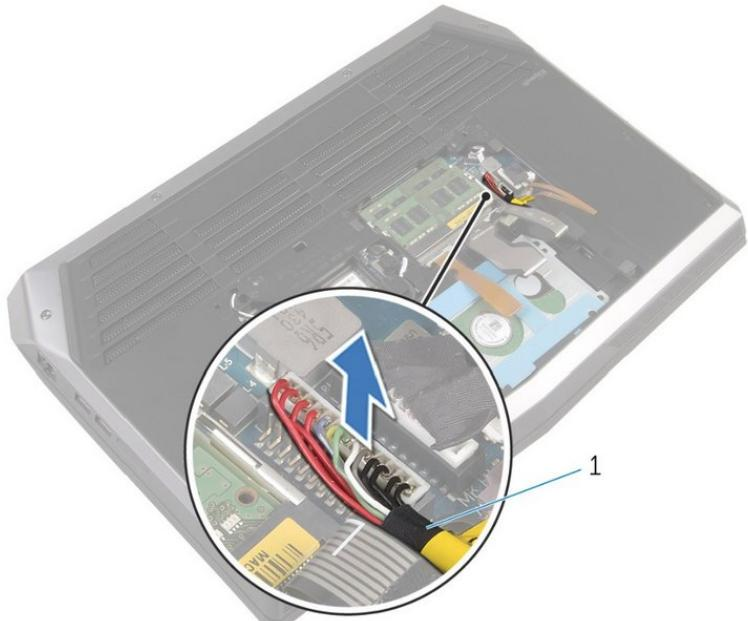
*(i)* You don't need to disconnect the laptop's battery if you are only replacing the back panel: only perform this step if you will be handling or replacing the electrical components of the computer.
