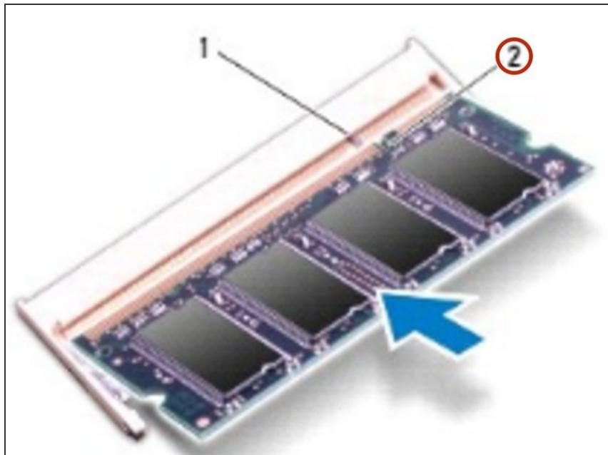
⚠ CAUTION: If you need to install memory modules in two connectors, install a memory module in the lower connector before you install a memory module in the upper connector.
