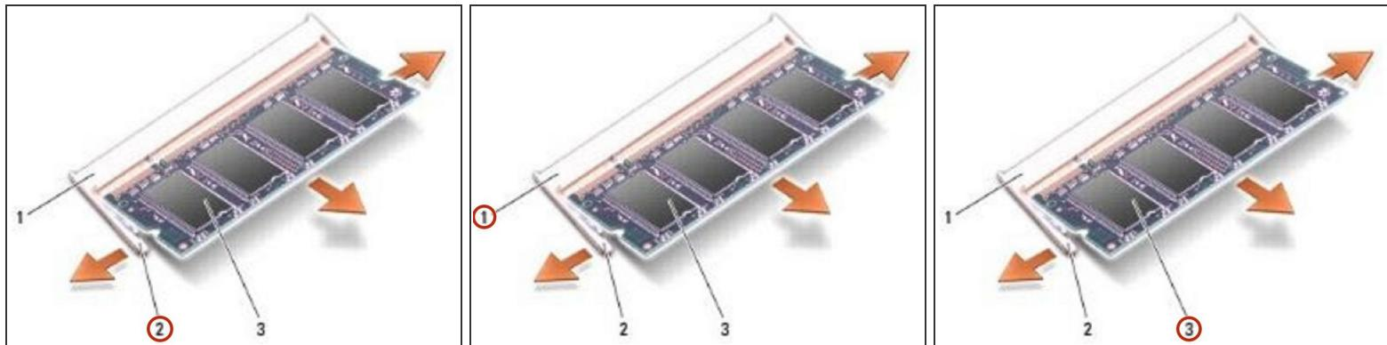
★ NOTICE: To prevent damage to the memory module connector, do not use tools to spread the memory module securing clips.
