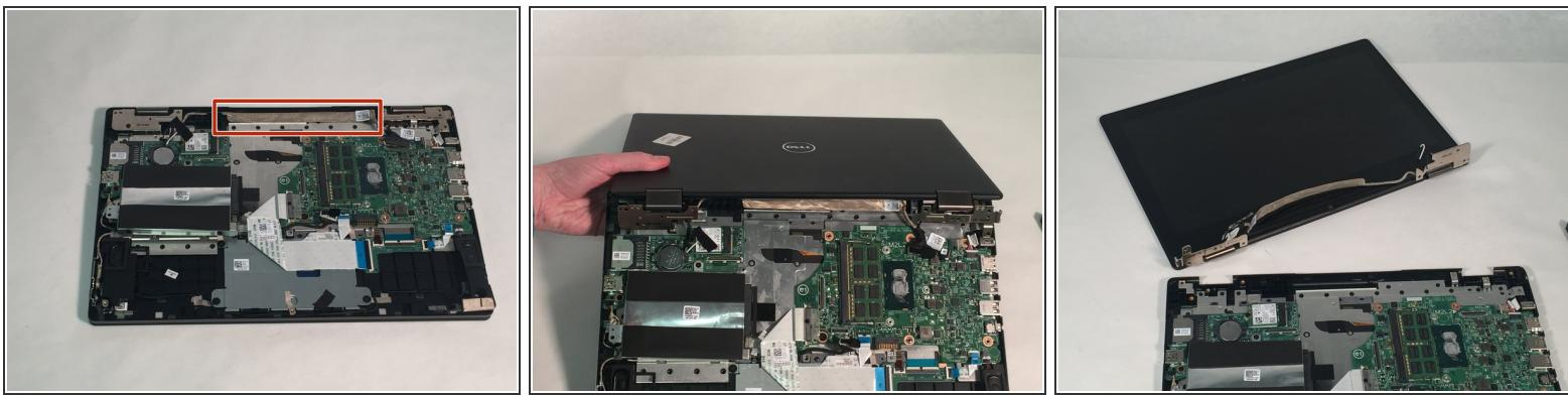
*(i)* Carefully remove the tape that is attached to the screen by prying it off with your fingers.
