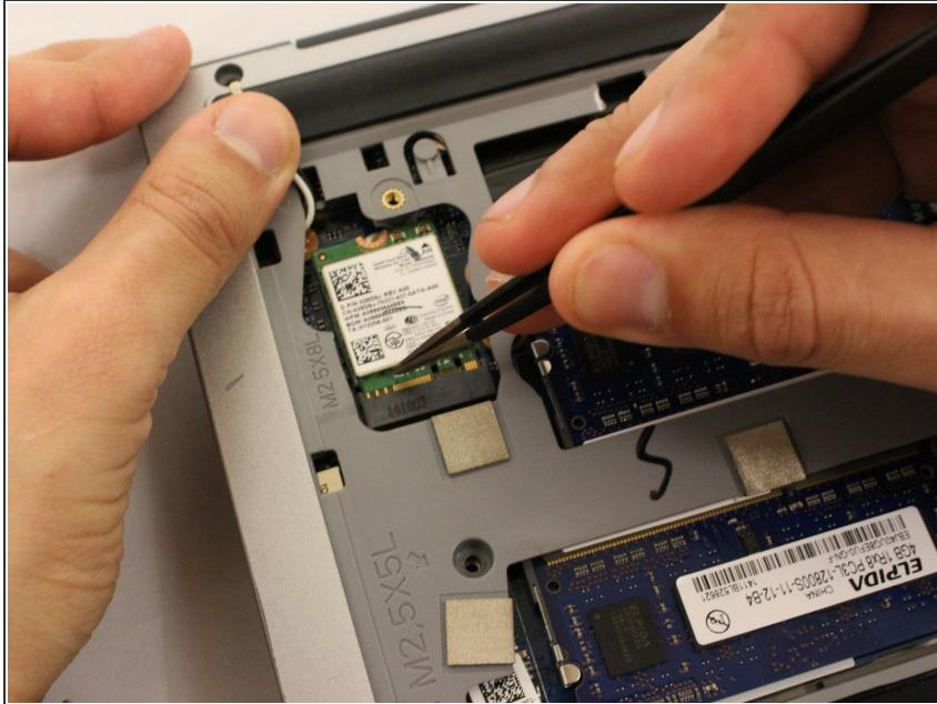
*(i)* The Wi-Fi card should slide out of the black socket.
