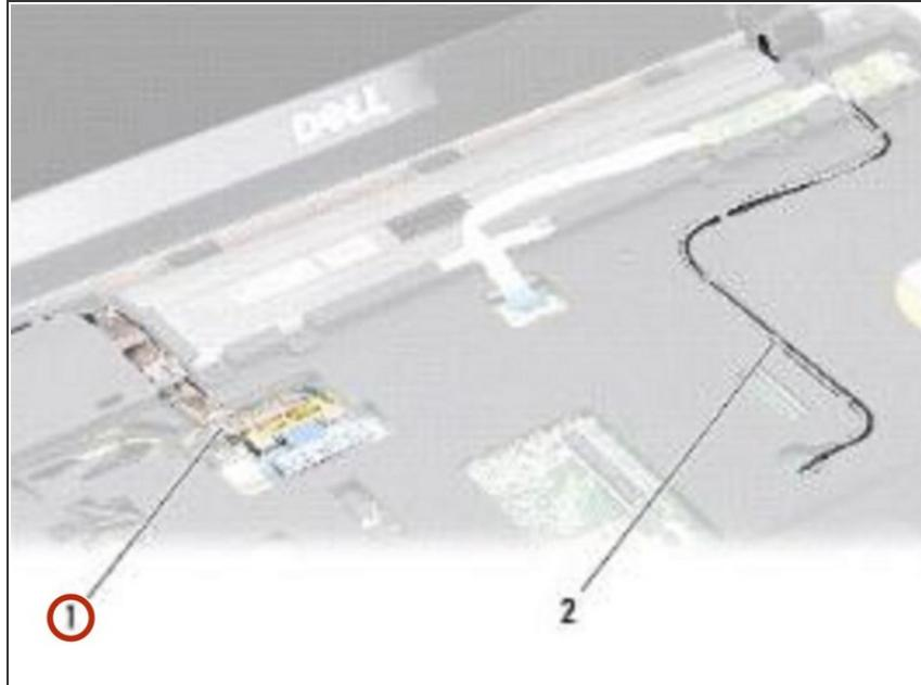
**i** NOTE: Note how the display cable is routed through their routing guides.
