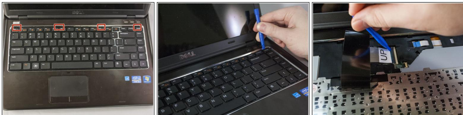
! careful lifting up on the key board once free there is ribbon connected to the bottom.
