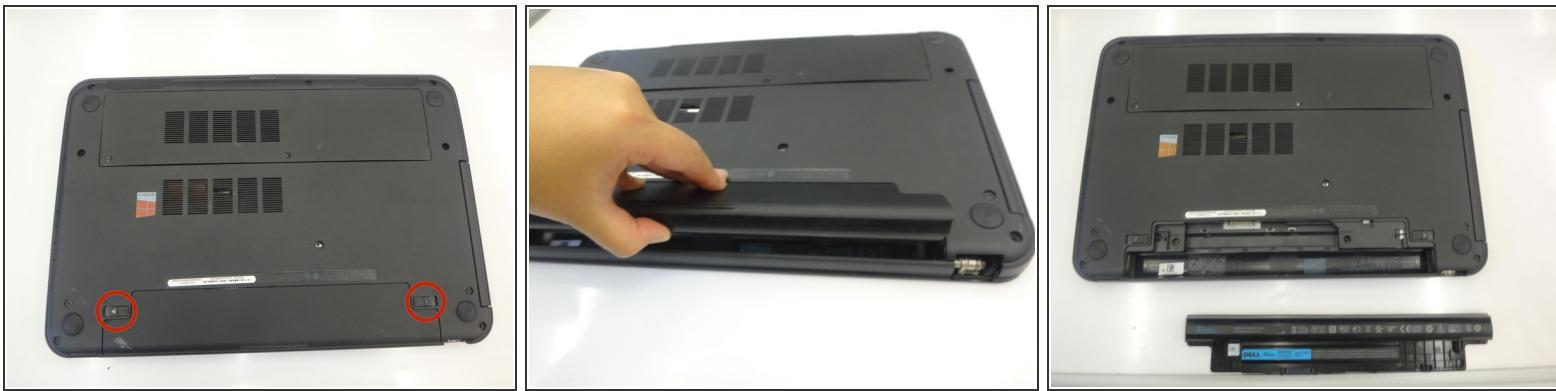
! We are removing the battery to avoid the possibility of an electrical discharge when working with this system.
