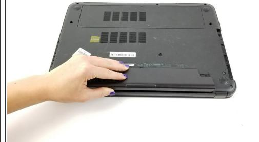
! Remove the battery to avoid electrical discharge while working with this system.
