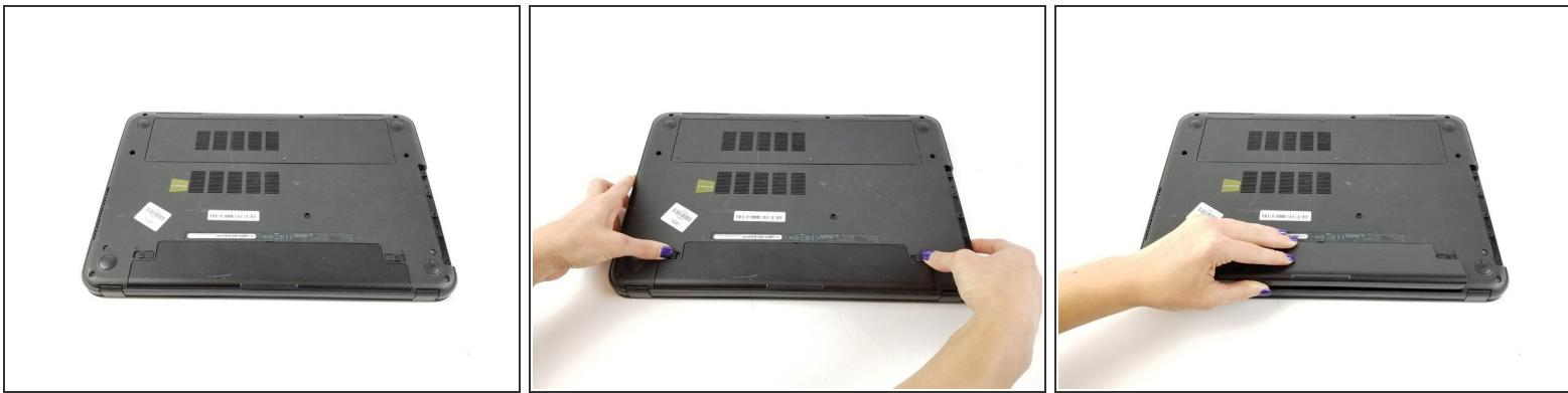
! Remove the battery to avoid electrical discharge while working with this system.
