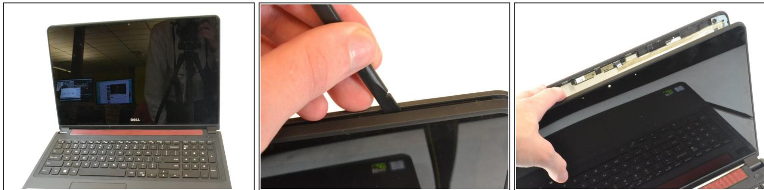
**⚠** This next step will likely cause some of the tabs, that hold the display, to snap. They will still function and hold the display in place and there should be no noticeable issues once put back together, but the tabs will have permanent damage and repeated disassembly will most likely require replacement.
