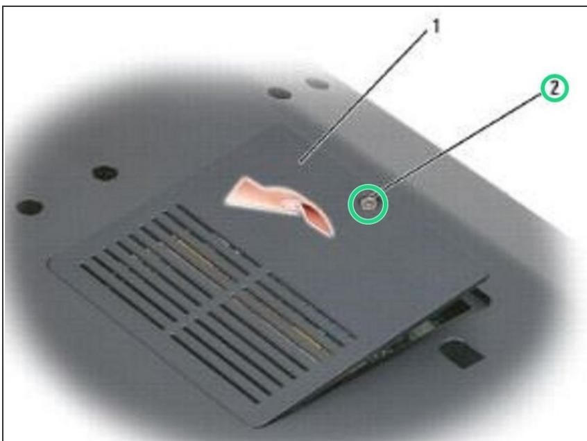
*★* NOTICE: If the cover is difficult to close, remove the module and reinstall it. Forcing the cover to close may damage your computer.
