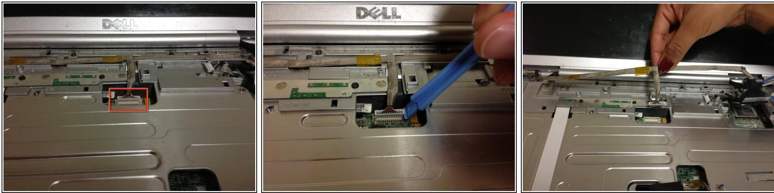
**⚠** When disconnecting the camera/microphone cable, pull up by the white plug. Pulling on the cable itself can damage it.
