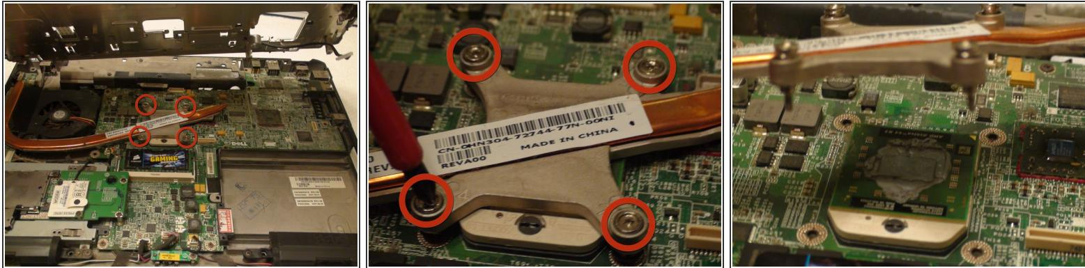
**i** The screws that hold the CPU heat sink in place are attached to the heat sink with springs and washers. They should only be loosened enough to detach the heat sink. Do not try to remove the screws from the heat sink itself.
