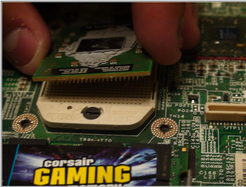
**⚠** The CPU has many small pins on the underside which can easily be bent. Bending CPU pins will permanently damage the CPU. Handle with extreme care to avoid bending any pins.
