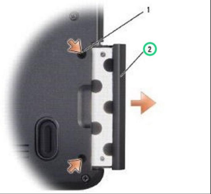
**NOTICE:** Use firm and even pressure to slide the hard drive into place. Excessive force may result in damage to the connector.
