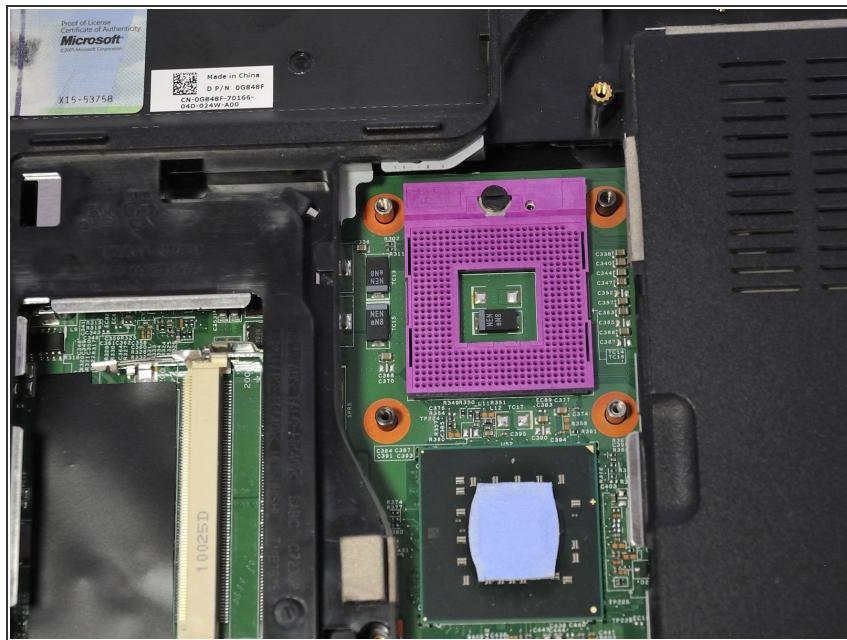
**⚠** The CPU is very fragile and has thin pins.
