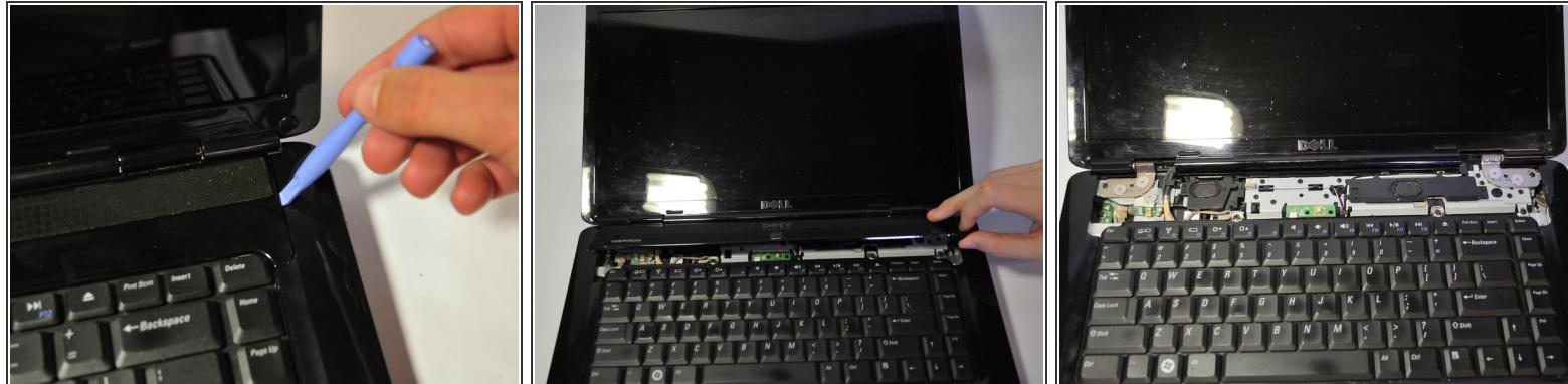
! The Center Control Cover is VERY fragile, be careful when using prying tools.
