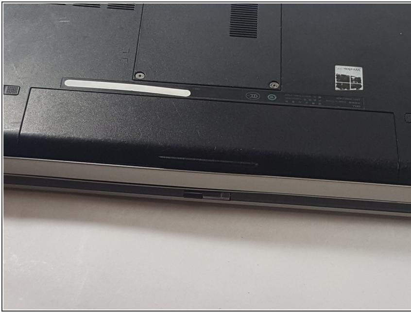
! We are removing the battery to avoid the possibility of an electrical discharge when working with this system.
