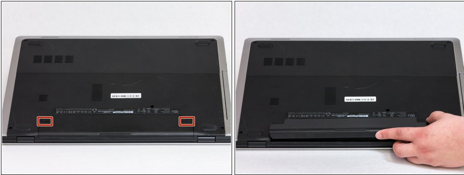
*(i)* First carefully turn the laptop over so you can access the battery.
