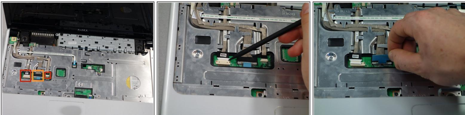
**⚠** Always pull wires from their plastic ends, not their cables, to avoid wire damage.
