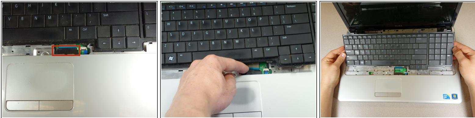
**⚠** Do not lift the keyboard completely free to avoid damaging its connections to the laptop interior.
