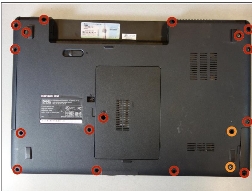
*(i)* Separate the screws by size and head type. Be sure to keep them in a safe place.
