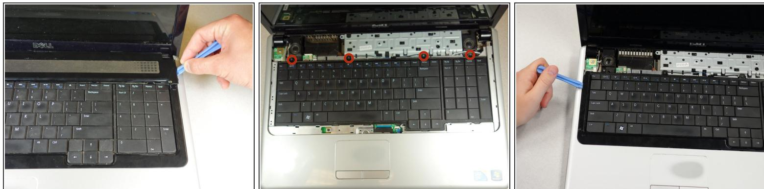
! Keep your hand pressed firmly on the back panel to prevent it from falling.
