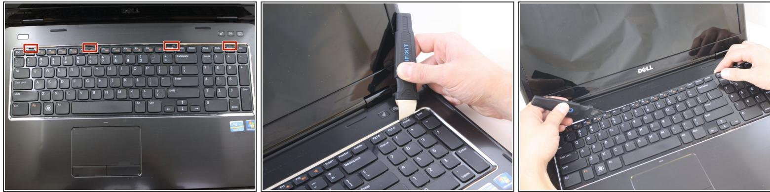
**⚠** Do not pull the keyboard away from the laptop. The keyboard is connected to the motherboard by a cable. Pulling the keyboard may cause damage to the keyboard and/or motherboard.
