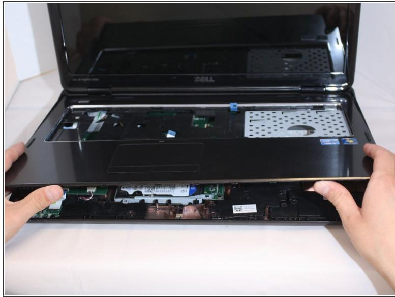
**⚠** Do not proceed without holding the laptop screen/lid for support. The screen is very heavy and may cause the device to fall if not held and supported.
