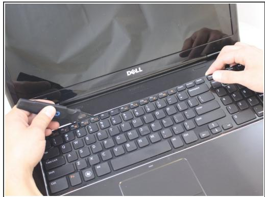
**⚠** Do not pull the keyboard away from the laptop. The keyboard is connected to the motherboard by a cable. Pulling the keyboard may cause damage to the keyboard and/or motherboard.
