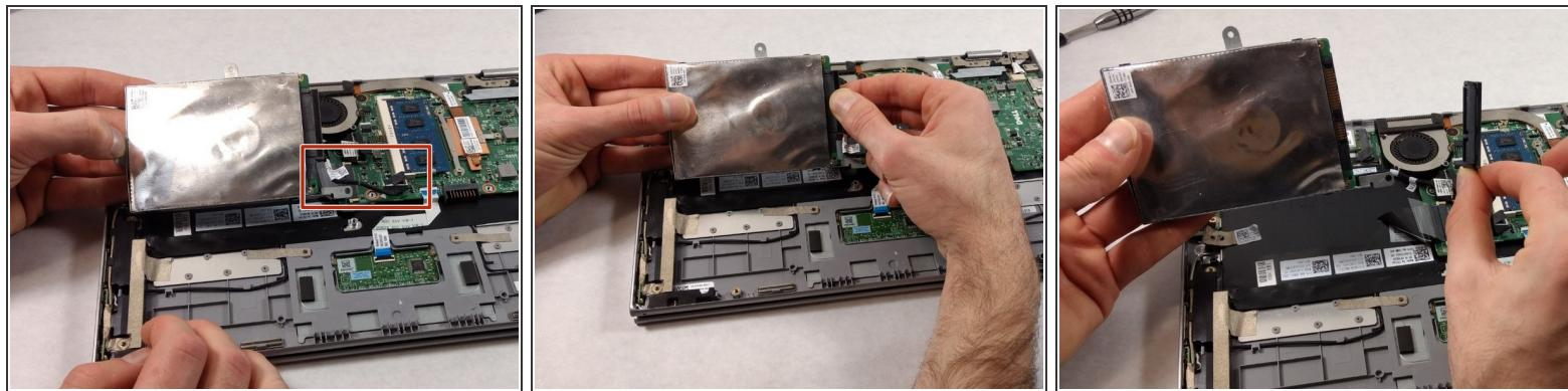
**⚠** Notice: there is a small data cable connecting the hard drive to the motherboard. Do not attempt to lift the hard drive all the way out before removing this cable.
