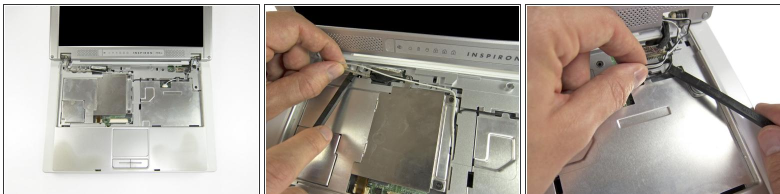
*(i)* There are four wires running from the display through small channels in the body of the 700m.
