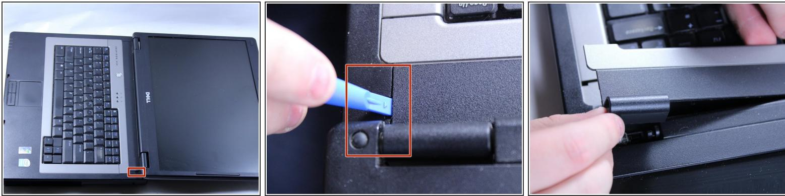
! When you pry the plastic plate off, be careful and pry gently so you do not crack the plastic.
