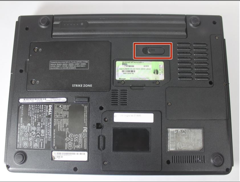
**⚠** Save your work, power the laptop off, and ensure that the charging cable is unplugged before removing the battery.
