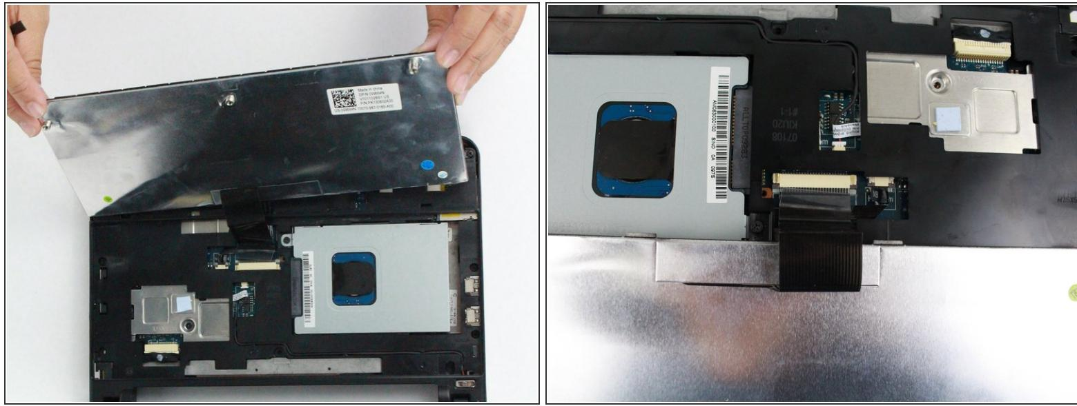
⚠ Lift the keyboard off of the support bracket carefully since it is still connected by a ribbon cable.
