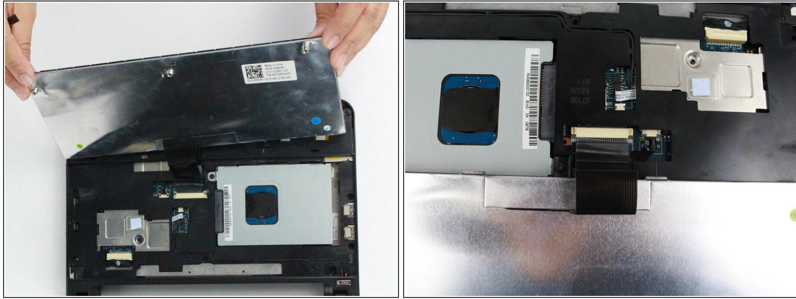
⚠ Lift the keyboard off of the support bracket carefully since it is still connected by a ribbon cable.
