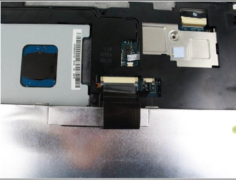
⚠ Lift the keyboard off of the support bracket carefully since it is still connected by a ribbon cable.
