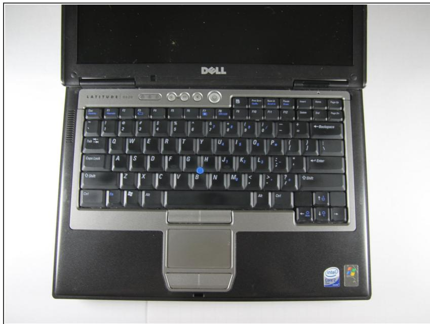
⚠ Power down the laptop and remove the battery.
