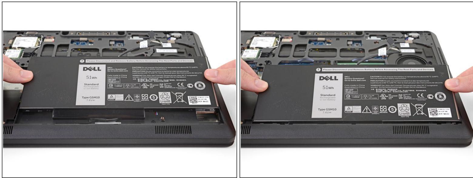
When installing your new battery, slide the bottom edge in first, and make sure it lays flat before you proceed to reinsert the screws or reconnect it.
